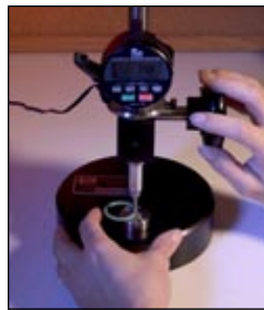
3) Verification of material hardness to Shore A or Shore M specification is completed on this gage.
