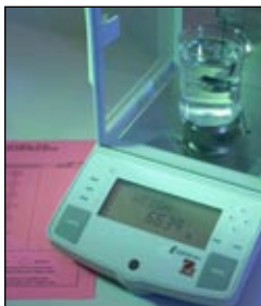
2) Specific gravity is used as a quality control tool, and for unknown samples, verification of material.
