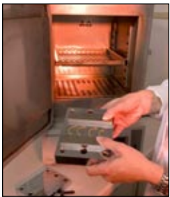
1) With the pictured oven and fixture, we can perform compression test on elastomeric materials.
