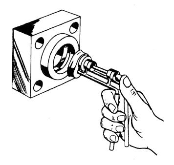
Available in three sizes: IT-100 for 1" to 1-1/2" shafts, IT-150 for 1-1/2" to 2" shafts, and IT-200 for 2" and up shafts.
