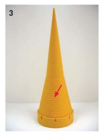
The raised numbers above the chosen cross-section slot will determine the "series" your O-Ring belongs to.
