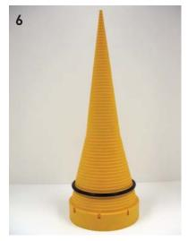
Read the O-Ring size from the step it is resting on. In this example, it is resting on the step between 428 and 430. Therefore, the size is 429.
