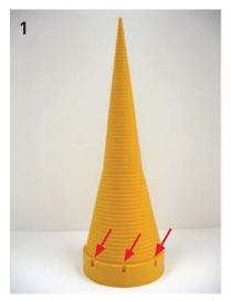
Locate slots at the base of the cone. This will determine the cross-section of your O-Ring.
